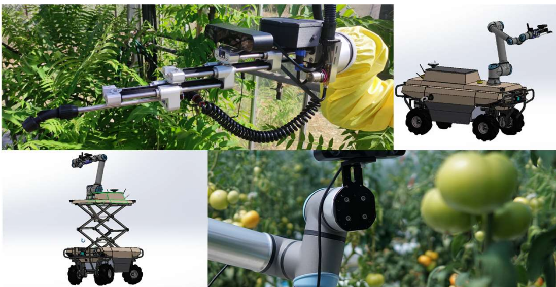
PestNu's autonomously navigated precision agricultural robot for greenhouses and the open field
